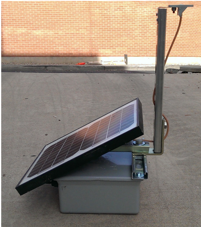
Fig. 1. Picture of the Saguaro INN. The solar panel that provides power to the unit and the sensor attached to the stalk are visible.
